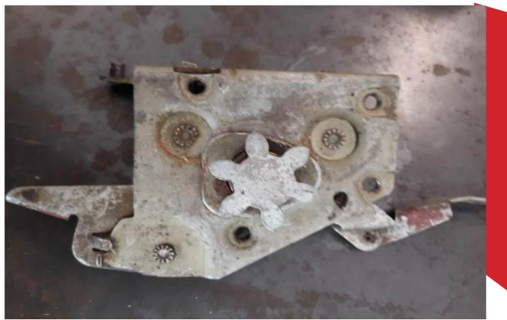
On the latch shown above, when I removed the phillips head screw and washer, I found that the star wheel was mounted on the end of the shaft with 2 "flats" ground onto the shaft, with the star wheel having a mating pattern. On mine, the flats in the shaft had been wallowed out of the years, which allowed the slop.
